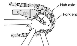
2. Place the non-turn washers onto the right side and left side of the hub axle. At this time, turn the cassette joint so that the projecting parts of the non-turn washers fit into the grooves of the fork ends. If this is done, the cassette joint can be installed so that it is almost parallel to the chainstay.
