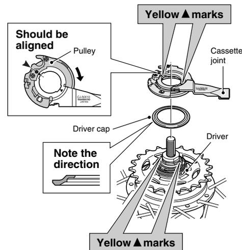
2. 1) Secure the cassette joint to the hub with the cassette joint fixing ring. When installing the cassette joint fixing ring, align the yellow ● mark with the yellow ● mark on the cassette joint pulley.
